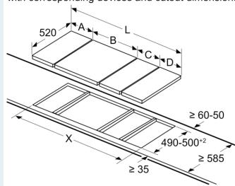
If two or more elements are installed right next to one another, one or several installation kits are required (2 elements 1 installation kit, 3 elements 2 installation kits, etc.).
