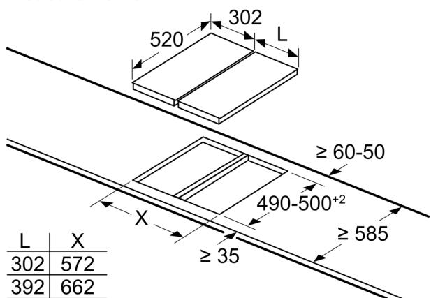
When installing two or more Domino units side-by-side, one or more assembly kits are required (2 units = 1 assembly kit, 3 units = 2 assembly kits, etc.).
