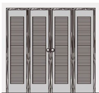
Double-folding louvered door: ventilation area 800 cm 2
