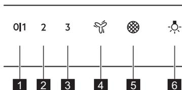
**1 First speed / Off** - The motor switches to first speed level. Second press turns off the appliance.
