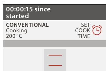
Once this phase has been finished, an audible signal will sound and the display will indicate that the oven has reached the set temperature.
