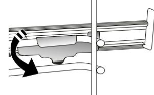
Please note: The sliding runners can be fitted on any level.
