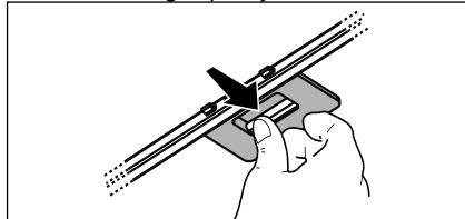
**NON-washable activated charcoal filter** - The saturation of the **charcoal filter** occurs after more or less prolonged use, depending on the type of cooking and the regularity of cleaning of the grease filter.
